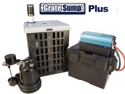
GrateSump Plus FastSump Pump 1/3 HP - 3 yr warranty (2400 GPH) w/ AC or DC power GrateSump Advance Sump Liner FastSump Power Inverter - 1 yr warranty 900w Inverter converts 12v DC to 115v AC 12v DC Battery - 1 yr warranty
